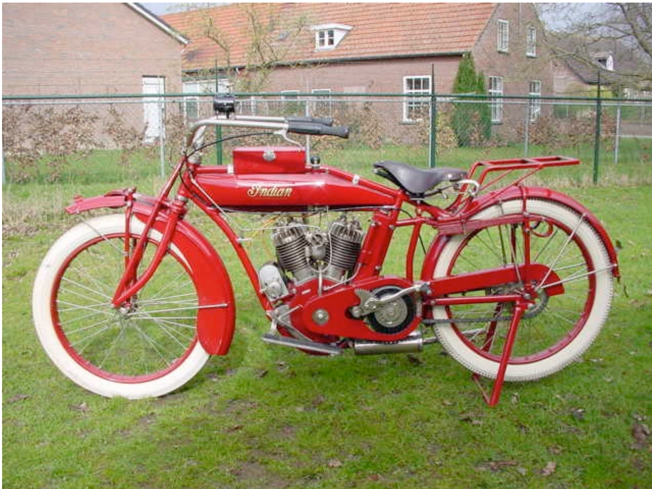
1916 Indian side valve "Powerplus" engine
